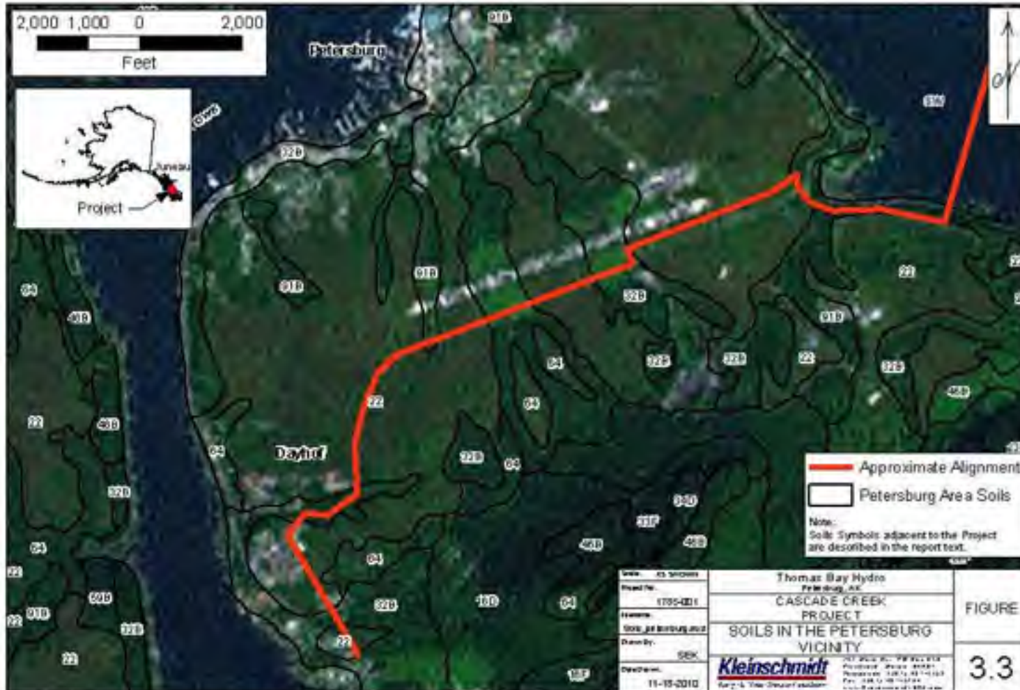
Figure 3-3. Transmission Line Across Petersburg Soils
